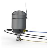
When the excitation locations are instrumented with external accelerom-eters, each location can be prepared with special M5 mounting studs. The shaker can then be used in a roving excitation setup to acquire FRFs from driveline and suspension interface locations.
